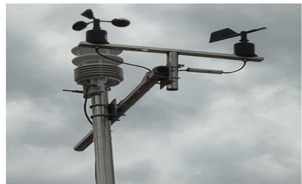
Figure 5. Smart Weather Sensor - Lufft type WS500-UMB
