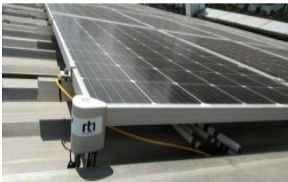
Figure 3. The RT1 irradiance sensor monitoring
